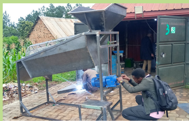
Local fabrication (using locally available and accessible materials) of the SUNSULA Maize cleaning equipment in Kampala, Uganda
