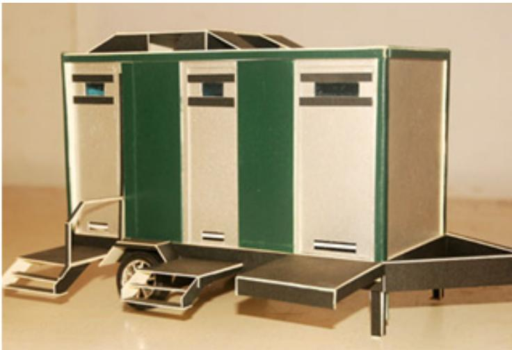
The smart portable trailer toilet will be constructed using metallic materials and will cater for the needs of disabled people. It will utilize solar energy in the functioning. Target deployment areas include suburbs with high water tables that make it difficult to construct pit latrines.
