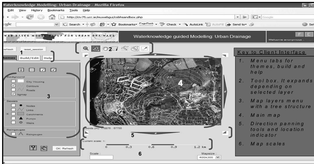
Figure 4: Web-GIS interface web-page dump for an urban drainage task
