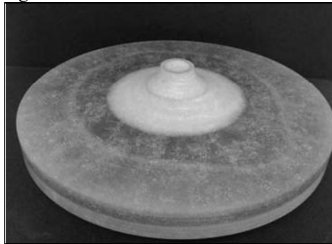
Figure 2: Complete hyperbolic profile using layered technique
