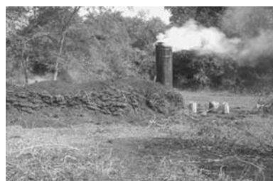
Figure 4: The kiln during carbonization
