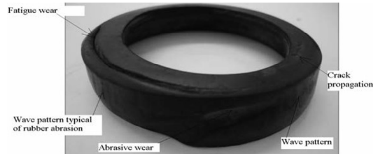
Figure 3: Indicators of fatigue and abrasive wear
