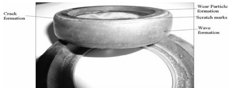
Figure 4: Indicators of fatigue and adhesive wear
